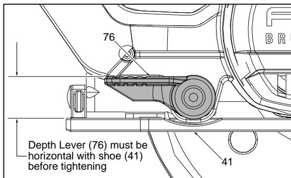
Depth Lever (76) must be horizontal with shoe (41) before tightening
