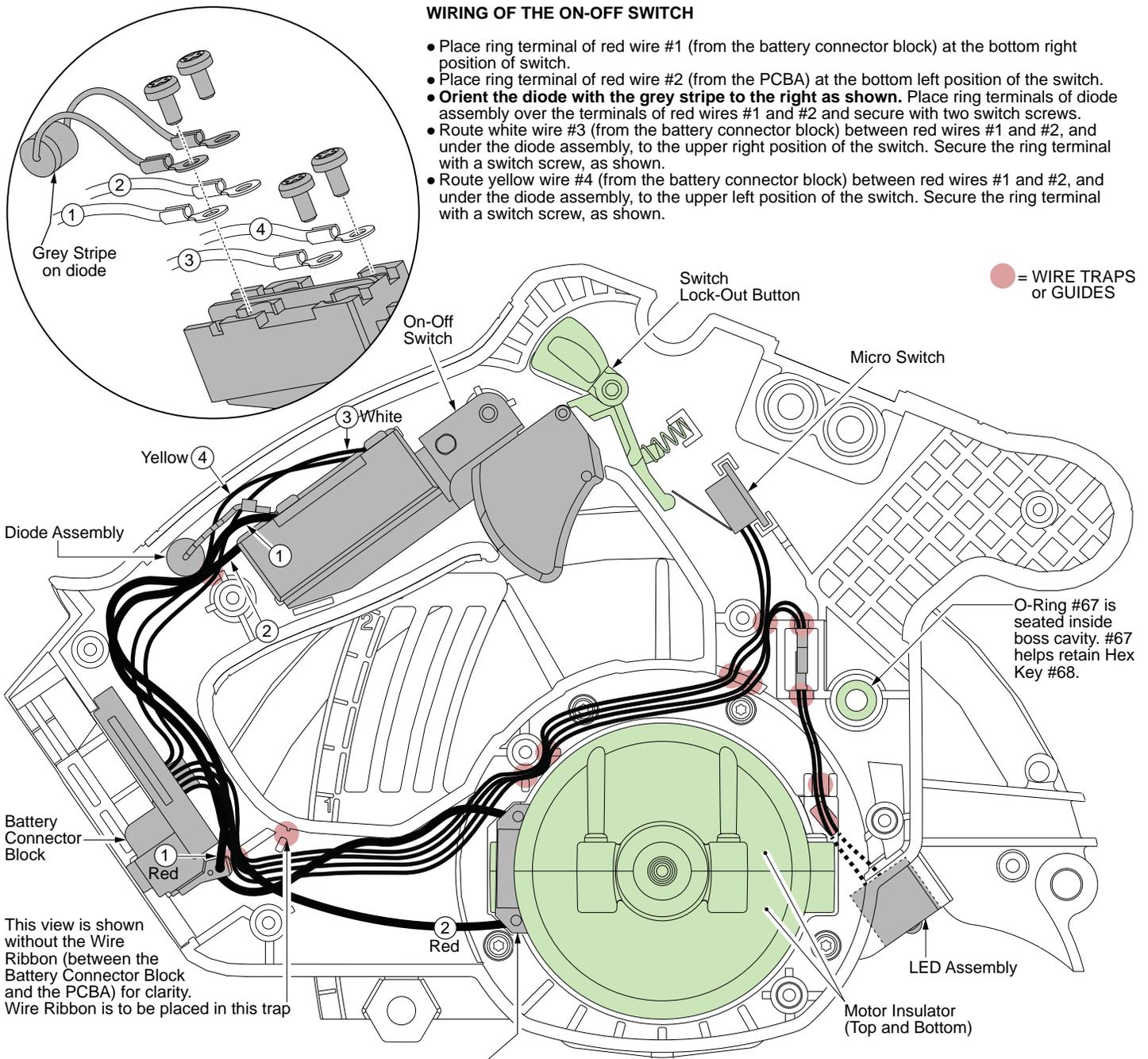
Stator / Electronics Assembly (Encased in the Motor Insulator Halves)
