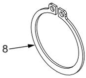
Retaining Ring (8) has a side with edges that are slightly rounded compared to the other side. When installing on the tool, position retaining ring with the rounded edge facing the lower guard.
