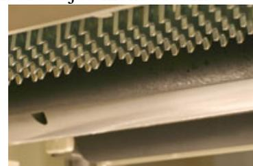
The anti-kickback fingers, rubber-covered feed rollers and the precision cutterhead make this machine safe and effective.
