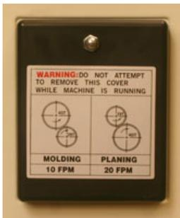
Behind the cover on the left is the feed rate gear set. Swapping these gears on their shafts changes the feed rate from 10 FPM to 20 FPM as shown on the diagram on the cover.
