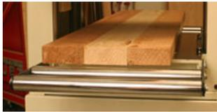
The main cast iron table and the twin-roller extensions add up to 36 1/2" of support that makes working with large pieces of wood much easier.
