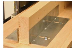
The optional Molding Guide Rail set (left) and Edge Guide Rail Set (right) make cutting profiles accurate, repeatable and safe.
