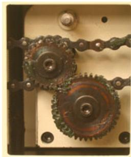
The JET 13" Planer/Molder has two feed rates, 20FPM (feet per minute) used primarily for dimensioning wood when lots of material is being removed quickly. 10FPM is used for finish cuts when the smoothest possible surface is desired. This slower feed rate is also used for molding operations.
