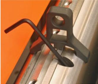
The straight planing knives are retained with gib bars, broken into three segments to accommodate the molding knives. A jack screw under each end of the planing knives and this easy to use knife height gauge make setting this machine up fast and simple.
