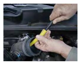
Install appropriate port adapter and insert smoke solution supply hose into adapter.
