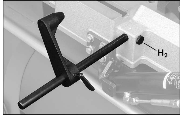
Figure 6-7: installing work stop (712 only)
