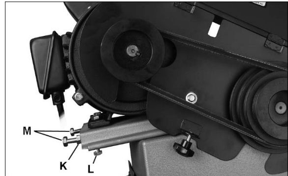
Figure 8-5: blade speed adjustment
