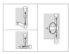
Hold the paint remover parallel with the surface of the workpiece. When presenting the tool, ensure that the planing base is in contact with the largest possible area of the surface.
