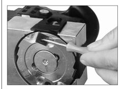
Scrape clean the Torx heads of the screws securing the reversible blades using the sharp-pointed tool (7).
