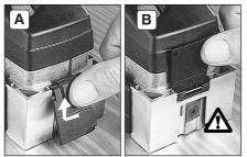
**A**: Open the protection flap as indicated and **B**: fold flap up into the fully-open position.
