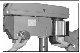
2. Slide the head stock opening onto the column.
