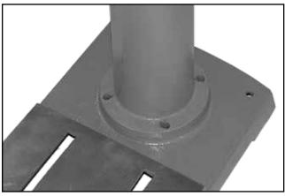
Align the mounting holes in the column with the corresponding holes in the base.
