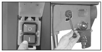
5. Turn ON the machine and adjust the speed.
