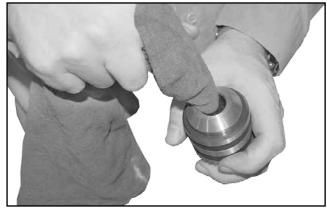
2. Clean inside the chuck with a dry cloth until all grease or lubricant is removed.
