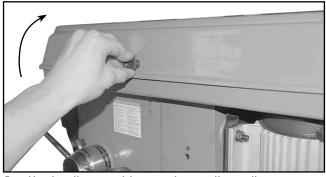
Unplug the machine, and open the pulley cover as shown.
