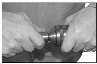
Make sure the arbor is inserted all the way into the chuck.
