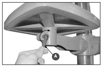
Lock the table in place by turning lever A clockwise.
