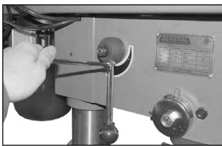
2. Tighten the handle using a 9 mm wrench.
