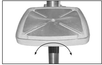
Till the table to the desired angle, and then retighten the nut A.
