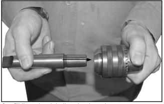
3. Fit the arbor into the chuck as shown.
