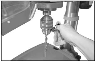
Secure the drill bit in the chuck by turning the key clockwise.
