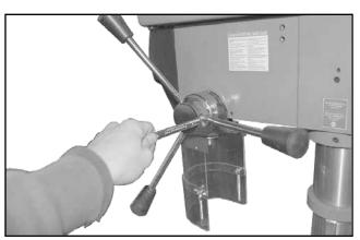
2. Tighten each handle using a 9 mm wrench.
