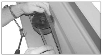
7. Slide the opposite end of the belt onto the other pulley, then turn the pulley until the belt snaps into place.
