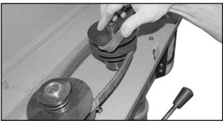
Slip a portion of the belt off and turn the pulley by hand until the belt comes off the pulley completely.
