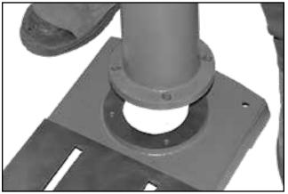
1. Set the base on a flat and stable surface, and then install the column on the base.
