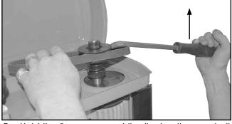
Hold the flange open while slipping the new belt onto the open pulley.
