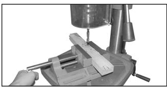
3. Secure the workpiece in a vise (optional).
