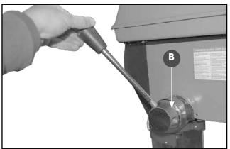
Thread the three downfeed handles into their mounting holes located in the support B.
