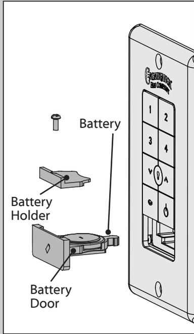
Before operating the wall control, press on the battery door to eject it. Unscrew the battery holder. Insert the battery, found in the control hardware bag, with the positive (+) side facing downward. Reinstall the battery holder and reinsert the battery door into the wall control.
