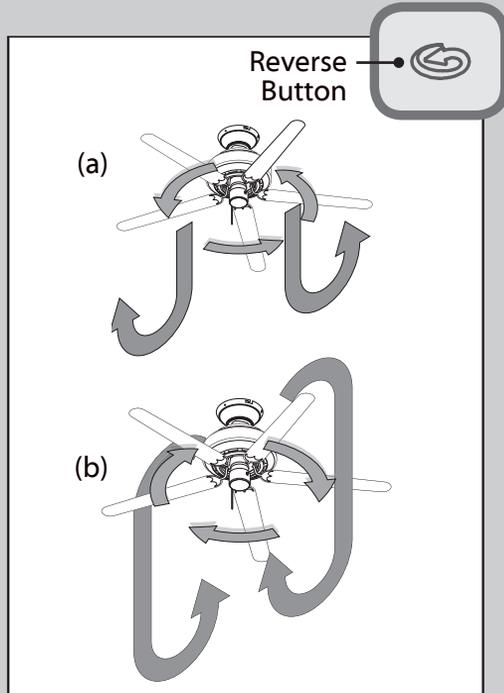
The reverse button on the wall control changes the air flow pattern. **In warm weather**, use (a) downward air flow pattern. **In cold weather**, use (b) upward air flow pattern.
