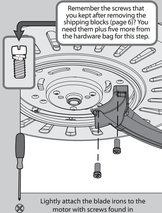
⊗ Lightly attach the blade irons to the motor with screws found in the ⊗ hardware bag, then securely tighten after both screws are attached.
