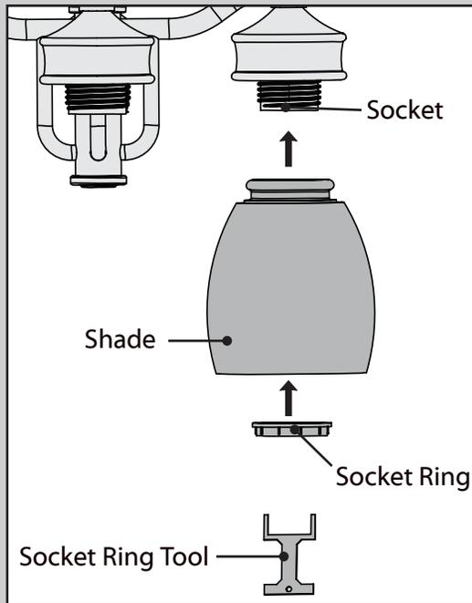
Remove the socket rings from the sockets. Install the shades onto the sockets. Install the socket rings onto the sockets. Tighten them by turning clockwise with the socket ring glass tool.
