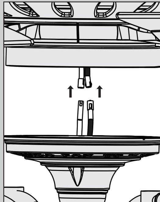
Connect the plug connectors between the black wire and the blue wire. Connect the plug connectors between the two white wires.
