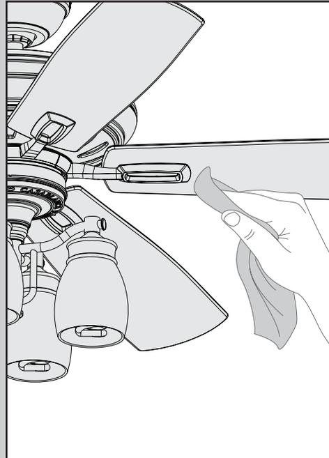
**Cleaning the fan** - use soft brushes or cloths to prevent scratching. Cleaning products may damage the finishes.
