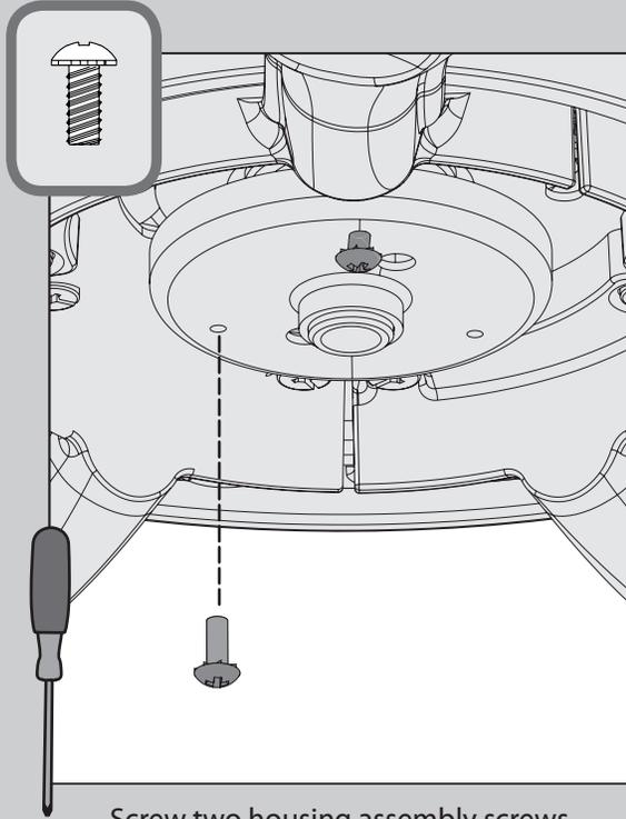
⊗ Screw two housing assembly screws from the
