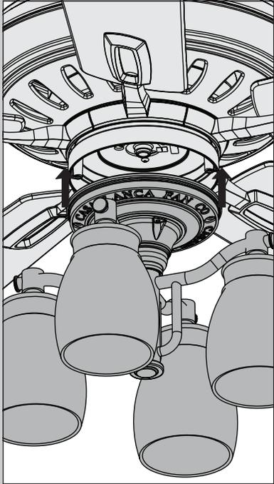
Lift the lower switch housing up until the holes line up with the screw holes in the upper switch housing.
