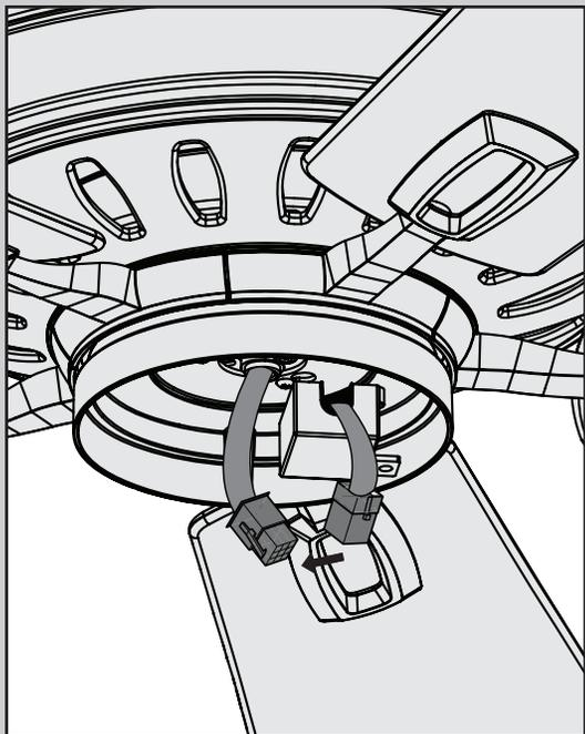
Connect the plugs from the motor and the switch housing. Make sure to line up the colored markings on the connectors.
