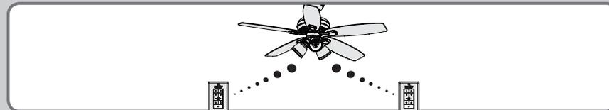
To have multiple remote controls operate one fan, you must pair each additional transmitter to the receiver in the fan. The transmitter that shipped with your fan is already paired.
