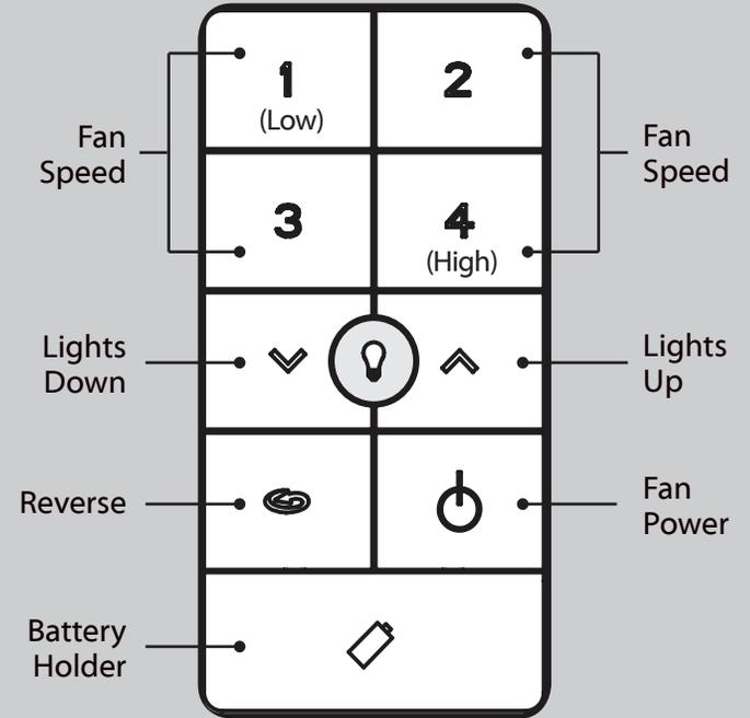
Quickly press the up or down arrow to turn the lights off and on. Hold the up or down arrow to dim or raise the light level. The reverse button changes the direction that the blades turn. The power button turns the fan off and on.
