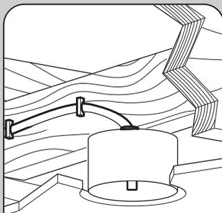
Must be able to secure the fan to building structure or fan-rated outlet box
