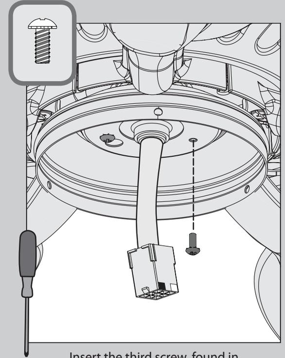
⊗ Insert the third screw, found in the
