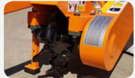
**9 Carbide Cutting Head - Direct Drive**
