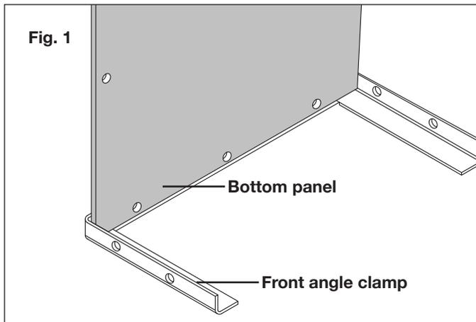
2. Push three M6 x 25 screws through the bottom panel and the front angle clamp. Secure the screws with flat washers and hex nuts, and tighten (Fig. 2).
