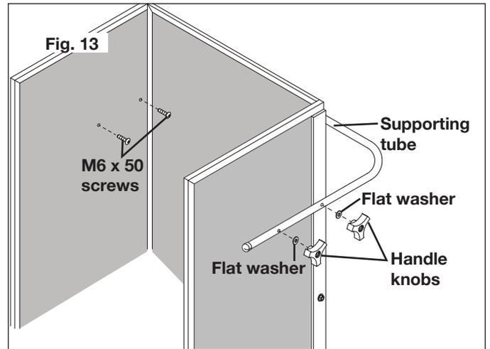
15. Place the handle tube over the side panels and line up the four holes. Assemble using four M6 x 50 screws through the side panels and handle tube. Secure with flat washers and handle knobs (Fig. 14).
