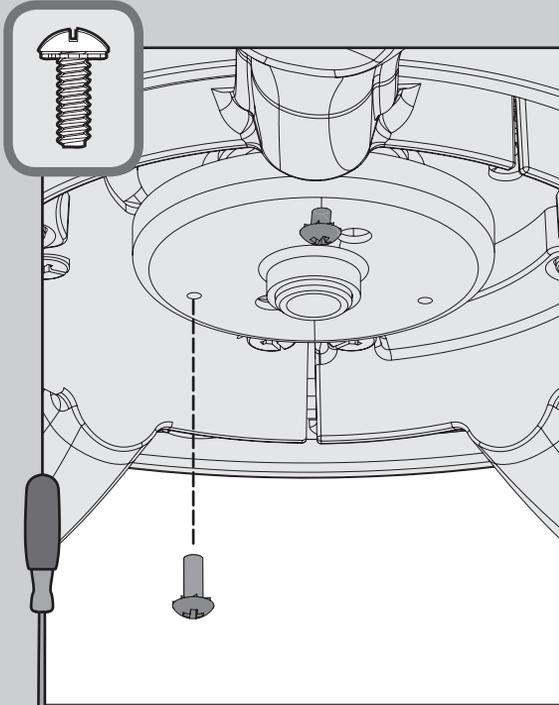
⊗ Screw two housing assembly screws from the
