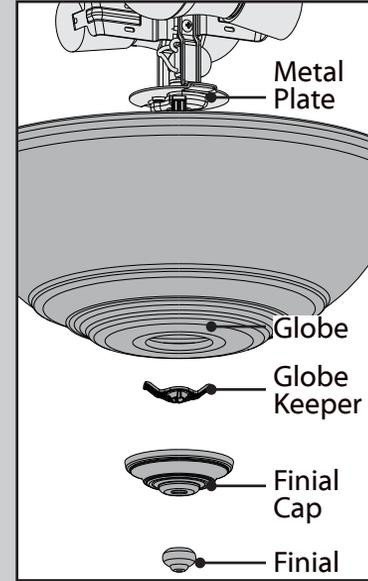
**Changing the bulbs** - unscrew the finial and remove it from the threaded rod. Remove the finial cap and unscrew the globe keeper while supporting the globe with your other hand. Carefully remove the globe. Unscrew bulbs and replace with bulbs of same type and wattage. Reinstall the globe assembly.
