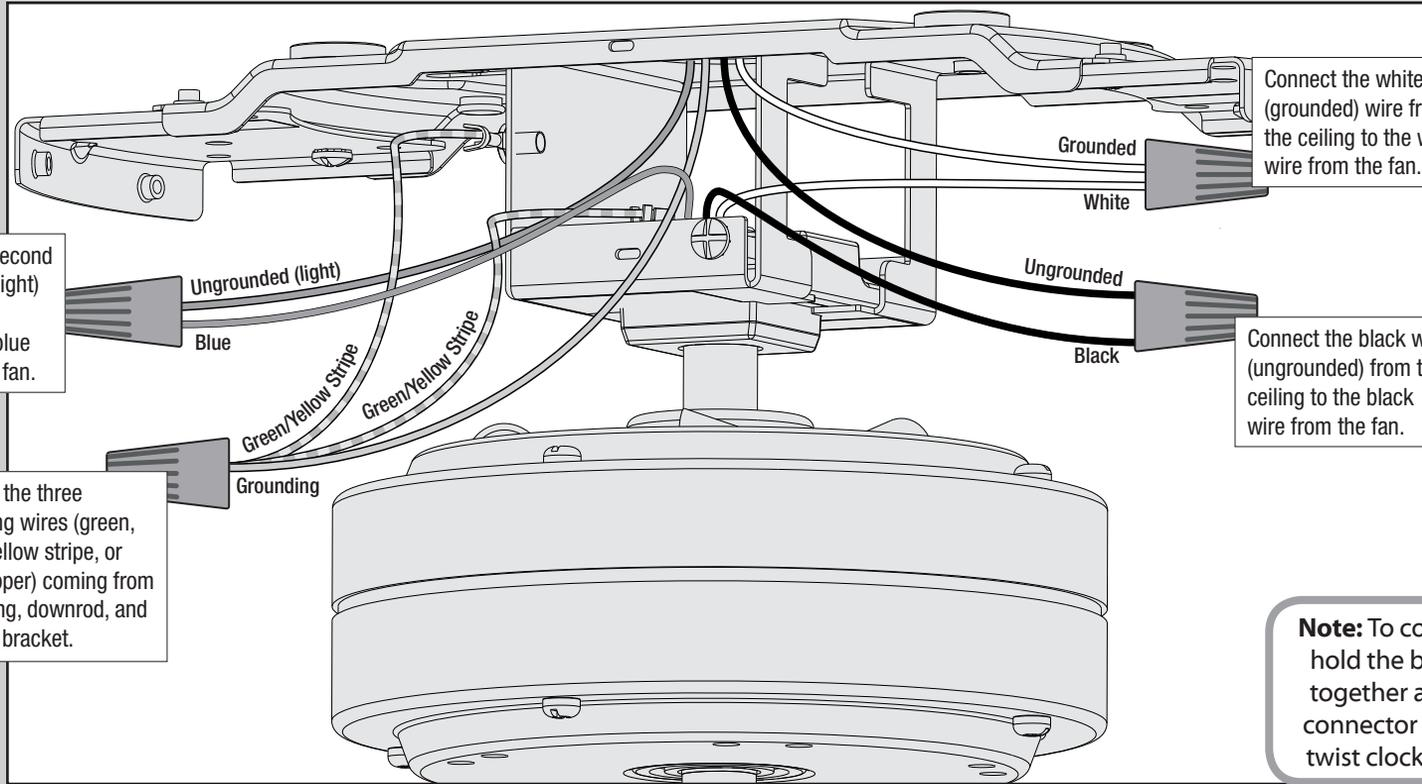
Connect the second ungrounded (light) wire from the ceiling to the blue wire from the fan.
