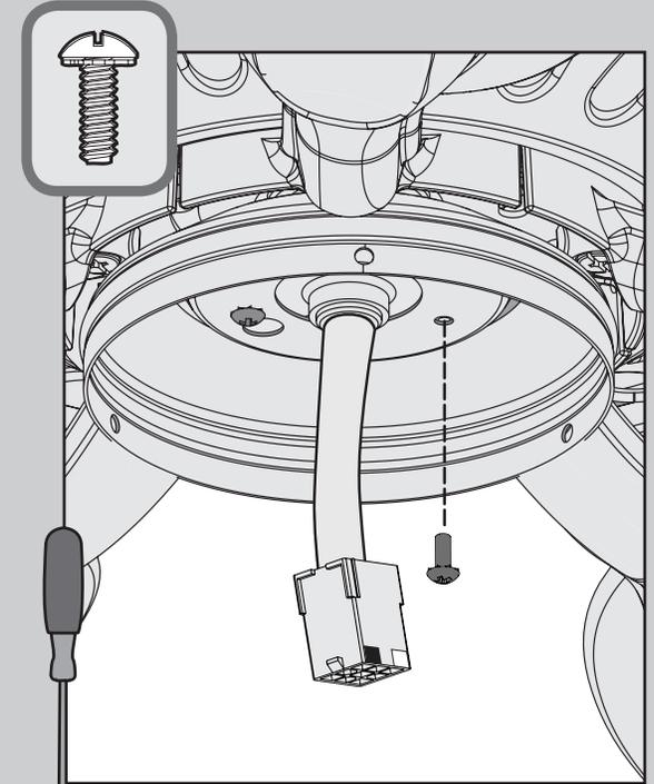
⊗ Insert the third screw, found in the
