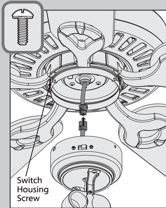
Partially install two of the switch housing screws found in the ☰ hardware bag. Connect the plugs from the upper and lower switch housings. Make sure to line up the colored markings on the connectors.
