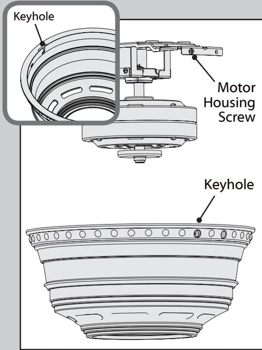
Lift the motor housing and align the keyholes in the motor housing with the two partially installed canopy screws in the hanger bracket. Rotate the fan housing to situate the screws in the end of the keyholes. **The motor housing is not secured until the next step is complete. Do not leave unattended.**
