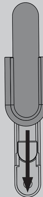
Slide the cradle onto the mounted bracket.
