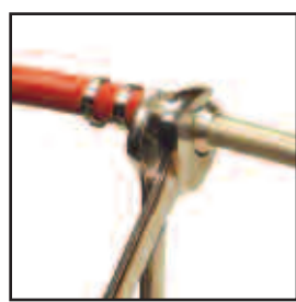
3 Tighten compression union onto aluminum line.
