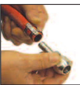
1 Place clamp onto hose, push adapter into hose.
