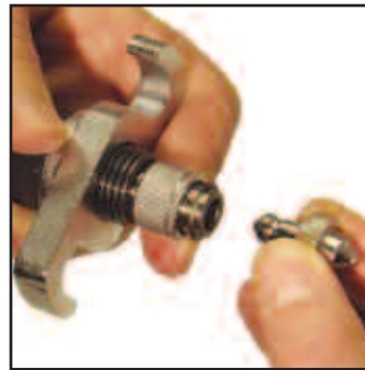
Quick Chuck for Fast Punch Changeover.
