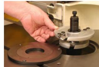
The full-height spindle (left) comes with various spacers that make securing cutters easy. The spindle is installed using the taper seat, a large lock nut and a drawbar. The height of the spindle combined with the spacious table opening (right) allow the use of large diameter cutters and even stacking cutters that are designed for that kind of operation.
