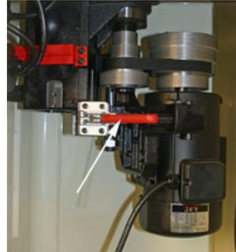
The entire motor mount and spindle assembly (right) is heavy-duty for maximum accuracy and durability. The belt tension release lever (arrow) makes changing speeds fast and easy.
