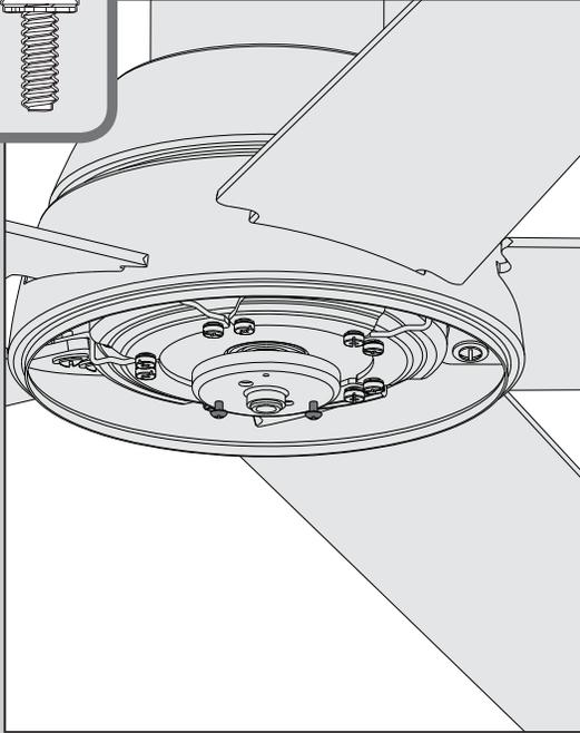
Partially install two light kit assembly screws, found in the
