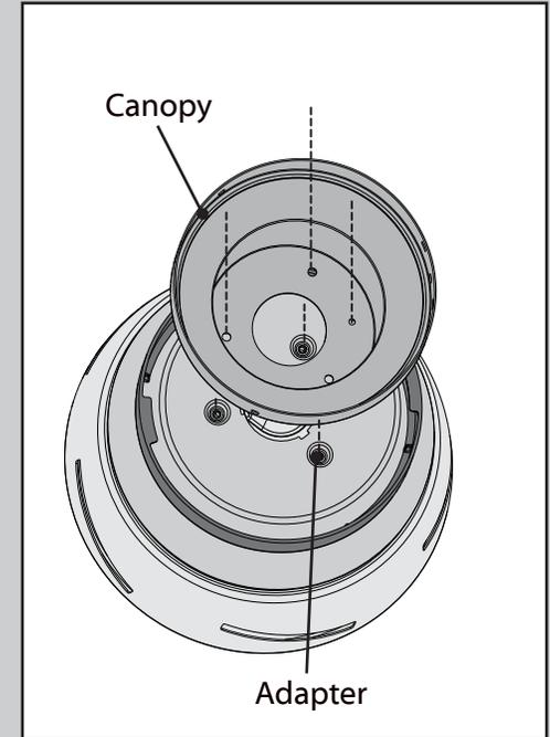
Place the canopy on the top housing. Ensure all four screw holes line up with the screw holes in both the top housing and the adapter.
