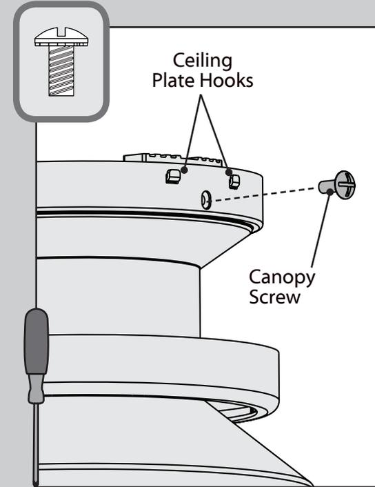
⊗ Partially install a canopy screw, found in the ● hardware bag, between the ceiling plate hooks. When all the holes are properly aligned, securely tighten all three canopy screws.
