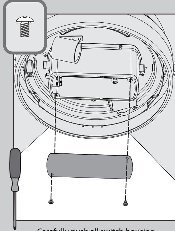
⊗ Carefully push all switch housing components into the switch housing, then install the switch housing plate using two light kit assembly screws, found in the ≡ hardware bag.
