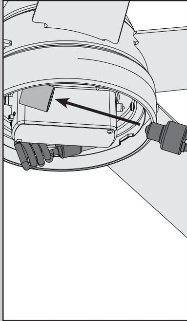
**Changing the bulbs** - carefully remove the globe. Unscrew the bulbs and replace them with bulbs of the same wattage. Reinstall the globe.
