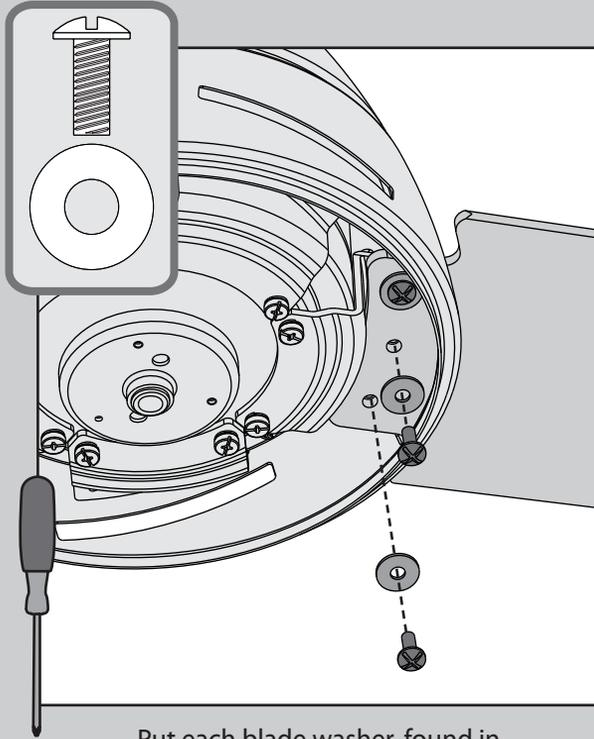
⊗ Put each blade washer, found in the ■ hardware bag, onto a blade screw, found in the ▲ hardware bag. Then secure each blade to a blade iron using the blade screws and washers.
