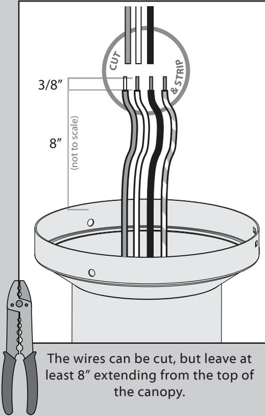
The wires can be cut, but leave at least 8" extending from the top of the canopy.
