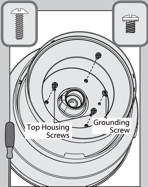
⊗ Install the top housing screws. Install the grounding screw in the smaller screw hole. These screws can be found in the ● hardware bag.
