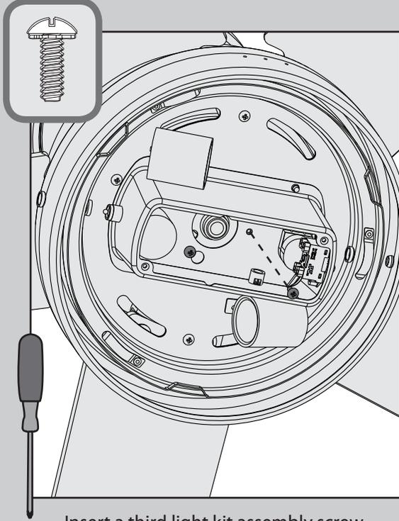
⊗ Insert a third light kit assembly screw, found in the ≡ hardware bag, into place and tighten all three screws securely.
