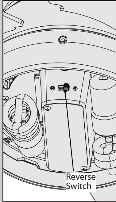
**Changing the direction of air flow** - carefully remove the globe and move the reverse switch to the opposite position. Reinstall the globe.
