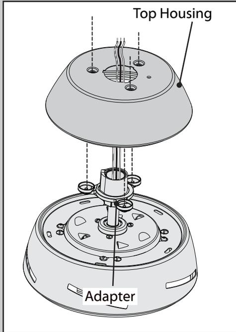
Thread the wires through the top housing. Place the top housing onto the motor housing so that the holes in the top housing line up with the holes in the motor housing and the adapter.
