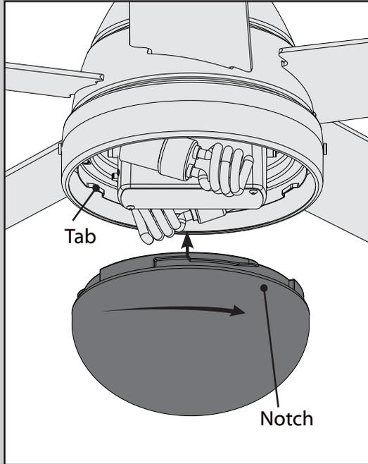
Align the notches in the outer rim of the globe with the tabs on the light kit assembly. Carefully lift the globe up inside the light fixture as far as it will go. Rotate the globe in a clockwise direction until it is held tightly in place by the three tabs.
