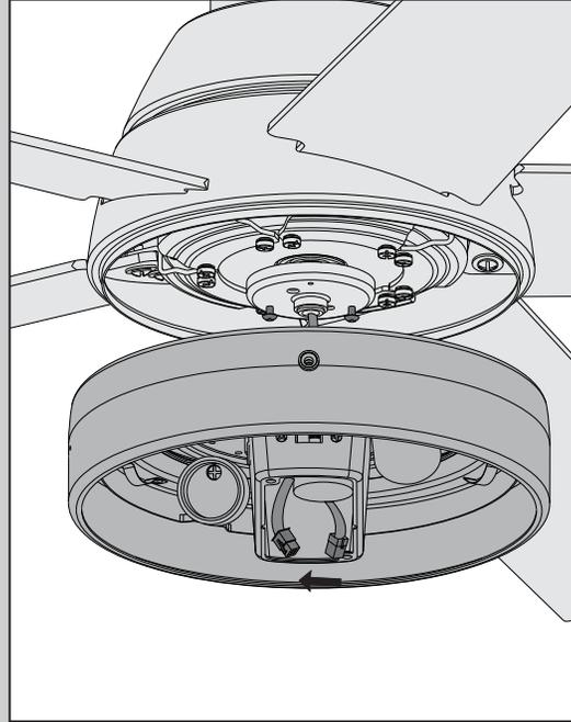
Feed the 9-pin plug connector coming from the bottom of the motor housing through the center hole in the light kit assembly. Connect it to the plug connector found in the switch housing area of the light kit assembly. Make sure to line up the colored markings on the connectors.
