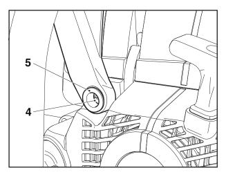
Remove the handguard and disengagement mechanism
