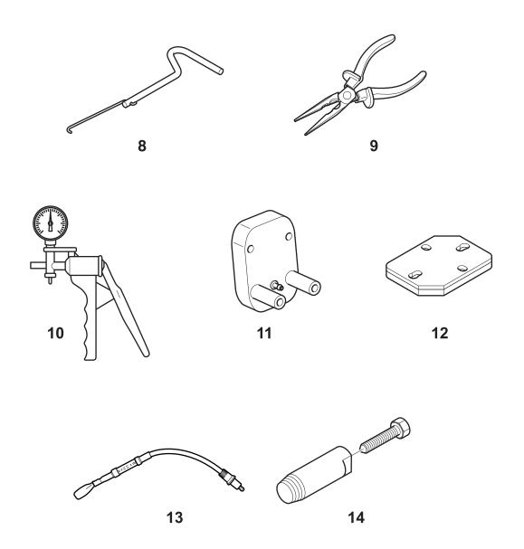
Disassembly hook Removal/installation **Brake band spring** 950.237.000 **Needle-nose pliers** Various assembly/ disassembly tasks 944.603.400 10 Over/underpressure pump For checking sealing of radial rings/carburetor 957.004.001 11 Sealing plate For sealing intake side 944.603.200 12 Sealing plate For sealing exhaust side 944.603.180 13 Ignition tester Checking the ignition 950.233.230 14 Radial ring puller
