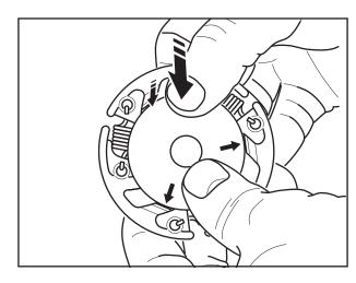
Press the disc onto the clutch. It must be flat and be engaged.
