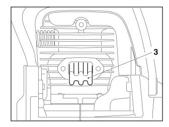
Move piston to bottom dead centre (visible through the exhaust opening).
