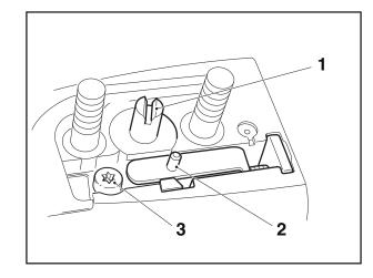
If necessary, turn adjusting screw 1 clockwise, until the fastening screw 3 is accessible.
