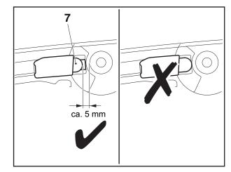
**Note:** Make sure that the handguard guide **7** is not unhooked. If necessary, push it back into position with a screwdriver (about 5 mm from the axle support). The handguard can only be assembled when the rest piece is in this position.
