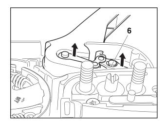
Remove the circlip 6.
