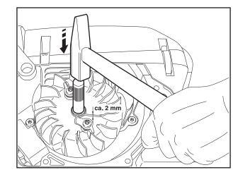
Screw the disassembly mandrel (chap. 00, Pos. 2) onto the threaded end of the shaft.
