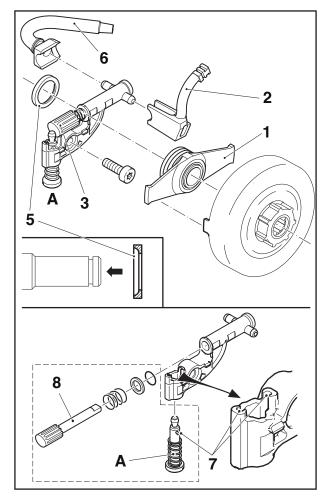
Pull the oil pressure line 2 from the oil pump. Unsrew screw **4** and remove the oil pump. Remove spacer ring **5** from the crankshaft.
