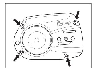
Remove the sprocket guard, bar, and chain.
