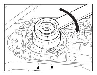
Insert wrench **4** (chap. 00, Pos. 6) into the clutch and use a socket wrench **5** to turn in the direction of the arrow (left-hand thread) to loosen and remove the clutch.
