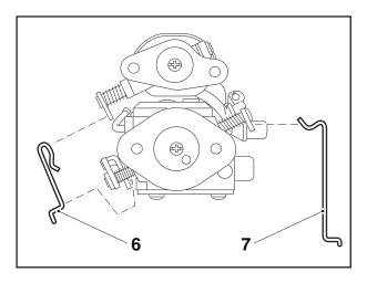
Before installing the air filter base, see Chap. 07 under **Combination switch**, and engage the choke linkage **7** in the choke valve actuator on the carburetor.
