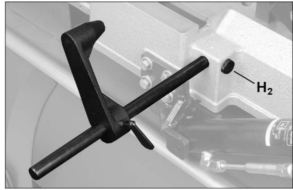
Figure 6-7: installing work stop (712 only)
