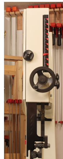
The upper guide post is operated by a rack and pinion drive that makes setting it simple and fast.
