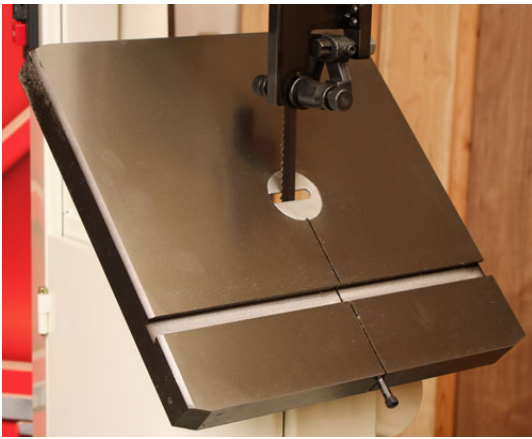
The tough cast iron table has a full-sized miter slot and tilts to 45-degrees right and up to 10-degrees left.
