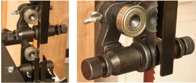
The upper and lower guide assemblies (left) are rugged and their adjustment tool free. Both assemblies use the popular European style carbide wheels (right) on either side of the blade.
