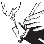
● Release E-Z Clear latch and open door. Remove jammed fastener. Close door and latch.
