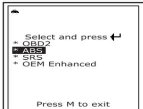
**To view SRS DTCs:** Select **SRS** from the System Menu (then choose the appropriate manufacturer if prompted). Refer to VIEWING SRS DTCs on page 51 to view SRS DTCs for your vehicle.
