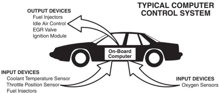
Vehicle operating conditions are constantly changing. The computer continuously makes adjustments or corrections (especially to the air/fuel mixture and spark timing) to keep all the engine systems operating within the preset reference values.
