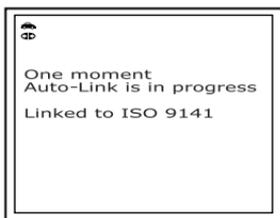
7. After approximately 10~60 seconds, the Diagnostic Tool will **retrieve** and **display** any Diagnostic Trouble Codes, I/M Monitor Status and Freeze Frame Data retrieved from the vehicle's computer memory.
