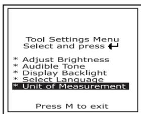
3. When the desired **Unit of Measurement** value is selected, press the **ENTER**
