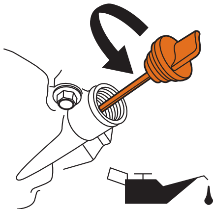
Figure 6 – Fill Engine Oil
