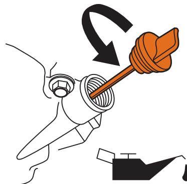
Figure 36 – Fill Engine Oil
