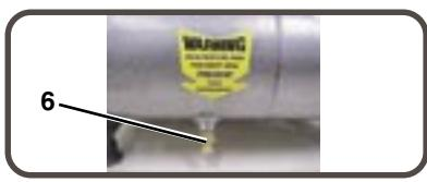
**6) AIR TANK DRAIN VALVE:** The drain valve is used to remove moisture from the air tank(s) after the air compressor is shut off. **NEVER attempt to open the drain valve when more than 10 PSI of air pressure is in the air tank!** To open the drain valve, turn the knob counterclockwise. Tilt tank to ensure that all condensation drains through valve.
