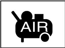
Never use oxygen, combustible gases or any other bottled gases as a power source for the Nailer.
