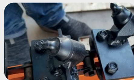
Tri-Cut High Carbide Teeth
