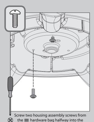
motor housing. It does not matter which
