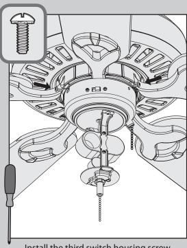
Install the third switch housing screw.
