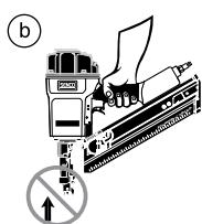
● The tool can be converted for non-toenail (flat surface) applications by adding the no-mar pad.
