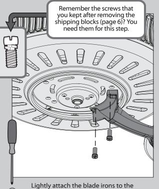
motor with the blade iron armature screws, then securely tighten after both screws are attached.
