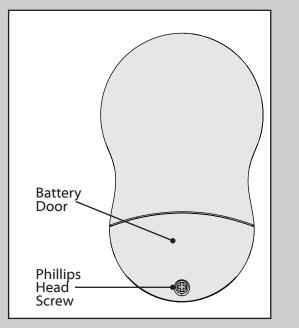
To access the battery compartment, remove the small Phillips head screw that secures the battery door to the transmitter assembly. The battery should be installed with the positive (+) side up. Replace with a CR2032 battery when necessary. If you are installing multiple remote-controlled fans on the same circuit breaker, you may need to perform a few extra steps to prevent interference or faulty operation of your remote controls.
