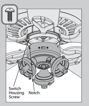
Partially install two of the switch housing screws found in the  $\equiv$  bag. Align the notches in the sides of the lower switch housing with the screws on the upper switch housing. Twist the lower switch housing clockwise to lock into place.
