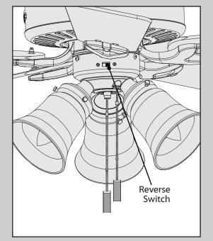
To switch the direction of air flow, move the reverse switch to the opposite position.
