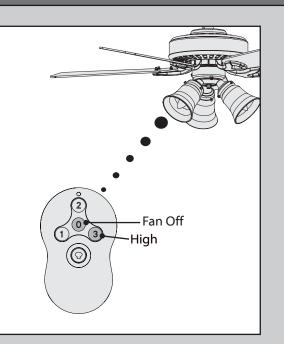
Note: The remote must be paired before the fan will operate. Within 3 minutes of restoring power to the fan, press both the Fan Off button and the High button for at least 4 seconds. Your fan will turn on low to indicate successful syncing. If it does not, turn off power to your fan, wait 1 minute then try again. If using the transmitter with multiple fans, repeat this process for each fan.
