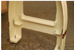
Even the legs are made from an iron casting and include these cast-in supports that make adding a shelf to storage area simple.
