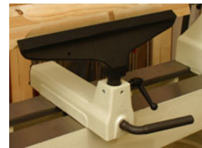
The 14"-long tool rest and its base are rigid and easy to reposition on the bed. The locking handle and mechanism make it easy to secure the tool rest assembly.
