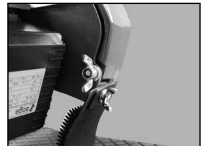
(R) Tighten the Blade Guard Pivot Point Retaining Wingnut.
