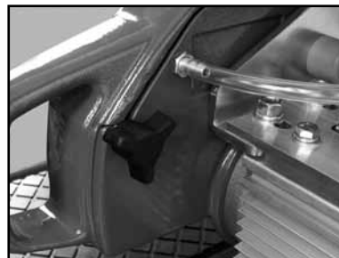
(Q) Tighten the Blade Guard Retaining Knob.
