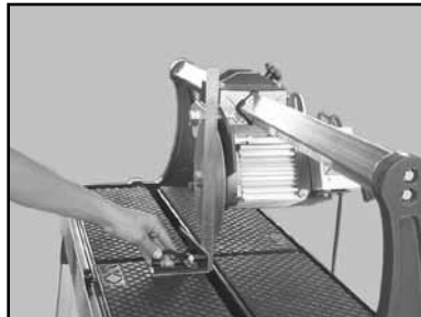
(B) Using a combination square, check the Blade for vertical alignment.
