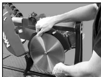
(I) Remove the old Diamond Blade.
