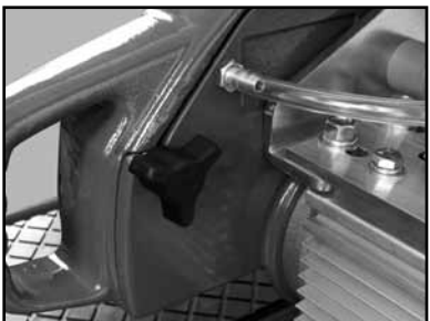
(G) Loosen the Blade Guard Retaining Knob.
