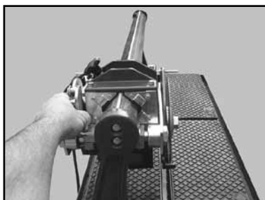
(G) Adjust the Guide Rail until it is aligned both vertically and horizontally.
