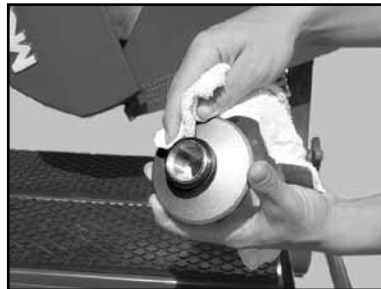
(B) Clean the Inner Flange.
