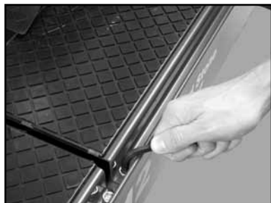
(D) Remove all Retaining Screws using the Allen Wrench provided.
