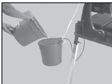
(D) Fill the external container until water completely covers the Water Pump suction.
