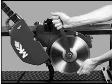
(A) Remove the Diamond Blade and Inner Flange.
