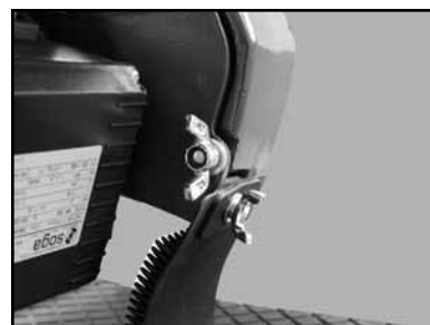
(F) Loosen the Blade Guard Pivot Point Retaining Wingnut.
