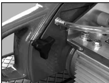
(E) Loosen the Blade Guard Retaining Knob.
