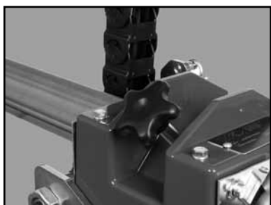
(A) Loosen the Cutting Head Locking Knob.
