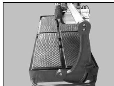
(C) Locate the table Retaining Screws on both sides of the cutting surface.
