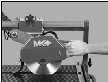
(B) Move the Cutting Head to one end of the saw. Tighten the Cutting Head Locking Knob.
