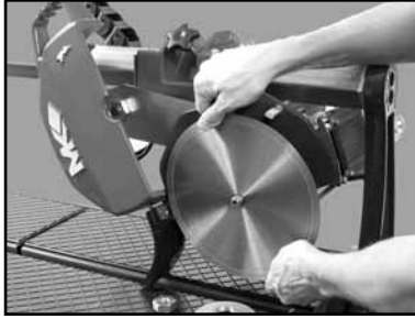
(K) Install Diamond Blade onto Blade Shaft
