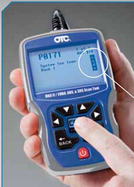
The CodeConnect® information takes vehicle repairs to another level. CodeConnect® provides actual fixes to the problem causing the check engine light to illuminate - providing the Top Reported Fix from the CodeConnect database. The Top Reported Fix is the most probable solution to the vehicle problem and is a shortcut for troubleshooting efforts.
