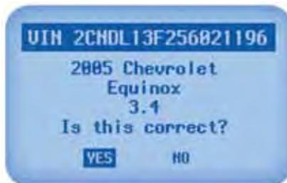
AutoID – Automatically pulls the VIN for most 2000 and newer vehicles and decodes to the vehicle make, model and year so you don't have to
