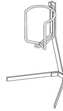
Gun holders are made to hold standard paint cups, gravity feed guns and cups, and paint filters.
