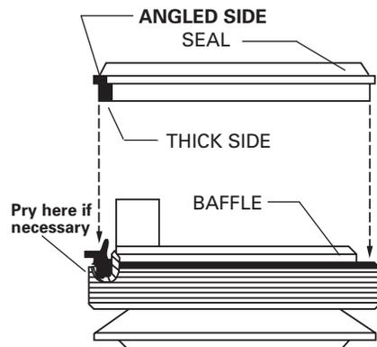
4. Assemble seal to baffle with **angled side up** as shown above. **NOTE:** The seal should be a tight fit on the baffle. If it is a loose fit on the baffle, assure that it is assembled with the angled side up.
