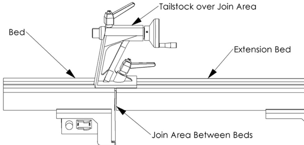
3. Move the tailstock until it is on top of the area where the Bed Extension face meets the Lathe Bed face (see illustration). The Bed Extension may need to be manipulated up, down or sideways in order for the tailstock to fit.
