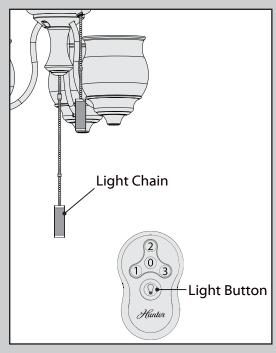
Push the light button on the remote transmitter. Pull the light chain once. If the light does not turn on, repeat step.
