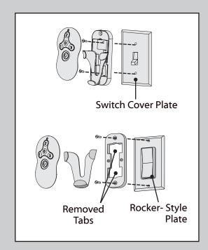
To install the transmitter cradle, remove the two screws holding the switch cover plate. Do not remove the cover plate. Orient the cradle by lining up the two mounting holes with those on the cover plate. Insert and tighten the screws. Do not over tighten.
