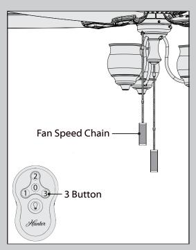
Push the 3 button on the remote transmitter for high fan speed. Pull the fan speed chain until the fan is on the highest speed.
