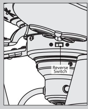
To switch the direction of air flow, move the reverse switch to the opposite position.
