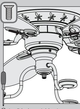
Install the three switch housing screws found in the ≡ hardware bag.
