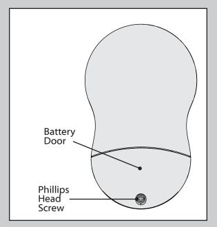
To access the battery compartment, remove the small Phillips head screw that secures the battery door to the transmitter assembly. The battery should be installed with the positive (+) side up. Replace with a CR2032 battery when necessary.
