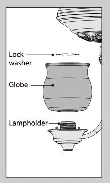
Place the globe over the threaded lampholder then install and hand tighten the threaded lock washer onto the lampholder.
