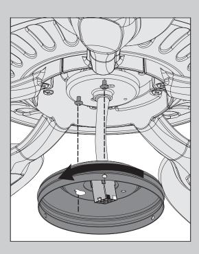
Feed the wire plug through the center hole of the upper switch housing, then wrap keyhole slots around the screws and twist counterclockwise.
