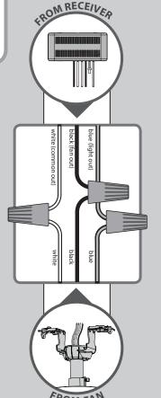
Using an orange wire connector from the hardware bag, connect the black wire (ungrounded) from the ceiling to the black wire from the receiver (marked "live in"). Connect the white wire (grounded) from the ceiling to the white wire from the receiver (marked "neutral in" or "common in").
