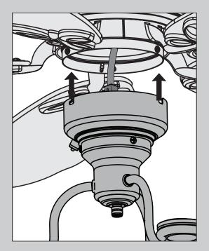
Lift the lower switch housing up until its screw holes are aligned with the screw holes in the upper switch housing.
