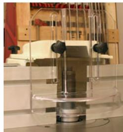
The table has a 7 ¼"-diameter opening for compatibility with the largest of cutter sizes. We also include inserts to reduce the table opening to 4 7/8" and 2 5/8". Mounted on the all steel base cabinet, the table surface is a comfortable 33 ¼" above the floor. A heavy-duty,
