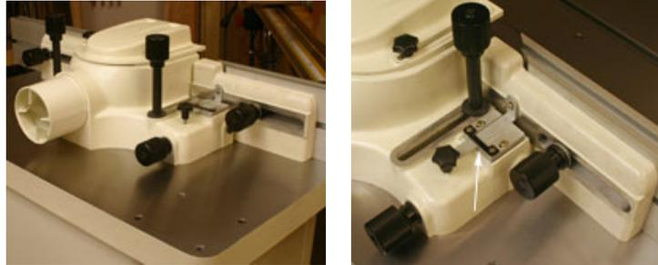
The left (operators view) fence half has a micro adjuster (front to back) for setting up ultra precise jointing operations. A gauge at its adjusting knob helps set the precise amount of offset desired for your jointing operation.
