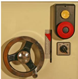
The controls on the front of the cabinet are easy to reach and use. The magnetic On/Off switch protects the motor and you. The large cast iron handwheel makes bit height changes fast and easy.
