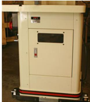
A large door in the cabinet side (left) provides easy access to the motor and belt system. It even has a large window through which the belt position can be confirmed.
