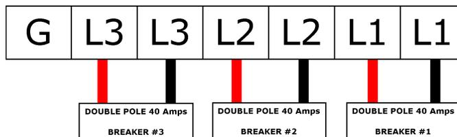
All wires must be connected to independent double pole breakers.
