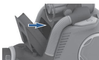
5. Refit the filter and filter frame back to the vacuum cleaner.
