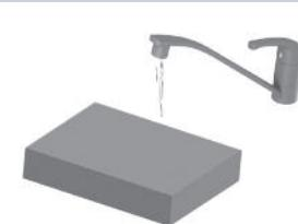
3. Wash the filter with cold water regularly or at least every 3 months. Filters should be replaced every 2 years (Ref. 118425501).
