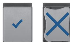
4. Squeeze the filter while washing. Let dry for 24 hours before fitting it back to canister. When the filter is dry, insert the filter into the filter frame properly without gaps.
