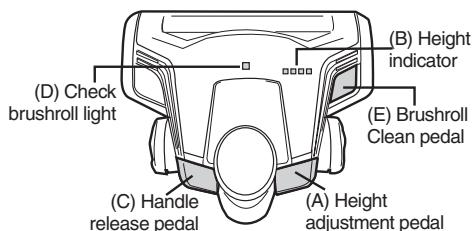
Do not use the Power Nozzle on the fringes of rugs without first turning off the brushroll.
