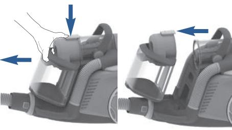
2. Release the dust cup by pushing the button on top of cyclone, and at the same time carefully pull the dust cup out from the canister.
