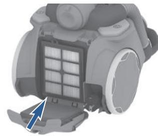
3. Let dry for 24 hours before placing it back to the canister. Replace the filter every 2 years.
