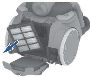
2. Remove the washable hygiene filter and rinse with cold water. Filter can be changed (EL012W).
