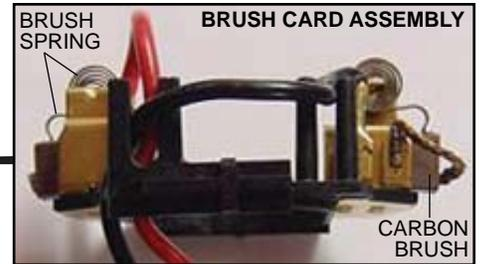
**IMPORTANT:** TO REINSTALL THE ARMATURE, CARBON BRUSHES MUST BE PULLED BACK IN BRUSH CARD ASSEMBLY. BRUSHES WILL BE HELD IN PLACE IN BRUSH TUBES BY PULLING BRUSH SPRINGS TO THE SIDE OF THE CARBON BRUSHES AS SHOWN. POSITION THE BRUSH CARD ASSEMBLY IN SLOTS OF LEFT HANDLE HALF (1A) BEING CAREFUL NOT TO INSERT COMPLETELY. ONCE ARMATURE IS PROPERLY INSTALLED, PRESS BRUSH CARD ASSEMBLY DOWN TO SNAP BRUSHES AND SPRINGS INTO PLACE.
