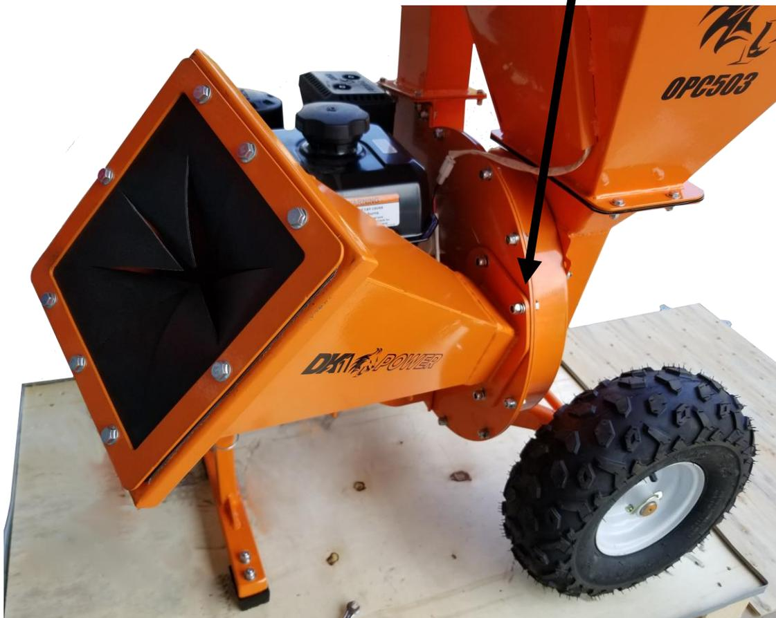
1. INSTALL THE HANDLE USING 4 BOLTS PREINSTALLED ON THE CHUTE FOR THE HANDLE TO BE ASSEMBLED.
