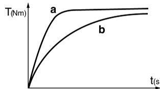
With an impact duration of approx. 5 seconds, the maximum tightening torque has been reached.
