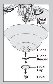
Press the globe and globe keeper flush against the metal plate. Thread the light pull chain through the hole in the center of the finial cap and thread the fan pull chain through the hole in the side of the cap. Finally, thread only the light pull chain through the hole in the finial and screw the finial onto the threaded rod.
