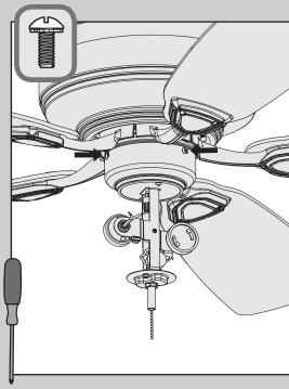
Install the third switch housing screw.
