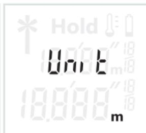
Switch off the measuring tool. Press the measuring button **1** and hold it down. The display will alternately show three units of measure. When the desired setting is displayed, release the measuring button **1**. The setting is saved.
