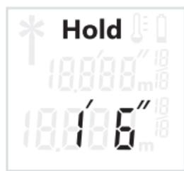
Press the "On/Off" button **1** to stop the measuring procedure. The laser beam is switched off and the **HOLD** indication appears on the display.
