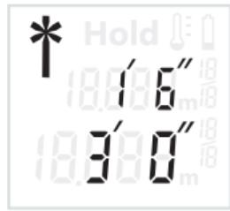
Press the "HOLD" button **1** once more to switch the laser on again. The laser indicator
