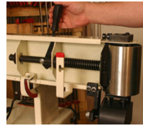
The rubber-coated drive drum (left) insures consistent, slip-free operation. The idler drum with its oscillating action and belt tensioning mechanism (right) make this a very effective sander.
