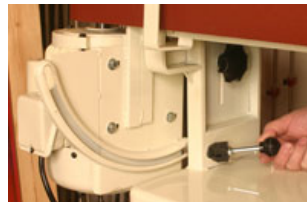
The ground steel platen has a graphite based covering (left) that keeps the belt moving smoothly. A single lever (right) allows tilting the belt system a full 90-degrees!
