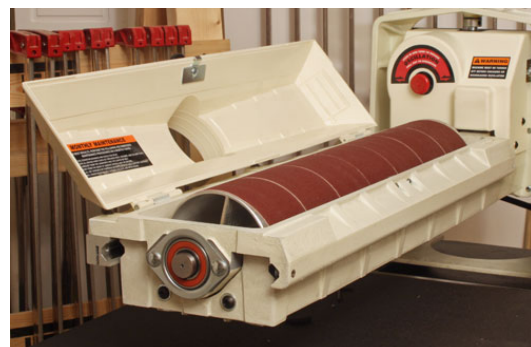
The sanding drum is precisely machined and balanced and then mounted in an exceptionally rigid arm to assure consistent accuracy.
