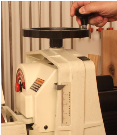
This large handwheel makes adjusting the drum height easy and very precise.
