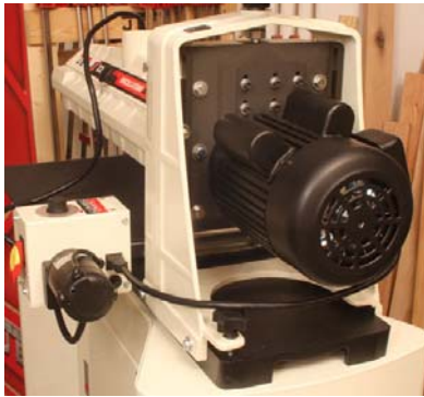
The strong, 1-3/4HP motor drives the sanding drum while a special DC-powered motor provides variable speeds to the conveyor belt.
