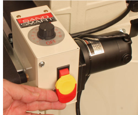
The variable conveyor speed control has our SandSmart™ technology built into it. When the loads at the sanding drum get to potentially damaging levels, the SandSmart™ system automatically takes over and slows the feed rate as needed.
