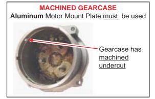
NOTE: Highlighted small tab of Motor Mount Plate (either NYLON or ALUMINUM) must-be-in-line with positive (+) terminal side of motor as illustrated to allow for correct placement of the motor and wiring in the handle of the tool A dab of red paint indicates positive (+) terminal
