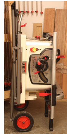
The JET Heavy-Duty 10" Jobsite Table Saw provides full-on table saw capabilities in its open mode (left) but makes transportation or storage far easier when the stand is closed. (right)
