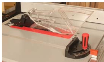
The blade guard assembly (left) is designed to work freely yet offer the best protection possible. When converted to the riving knife configuration (right), this system makes grooving-type cuts much safer and helps prevent kickback.
