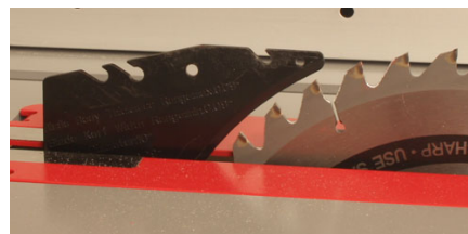
The blade guard assembly (left) is designed to work freely yet offer the best protection possible. When converted to the riving knife configuration (right), this system makes grooving-type cuts much safer and helps prevent kickback.
