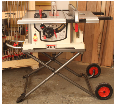
The JET Heavy-Duty 10" Jobsite Table Saw provides full-on table saw capabilities in its open mode (left) but makes transportation or storage far easier when the stand is closed. (right)
