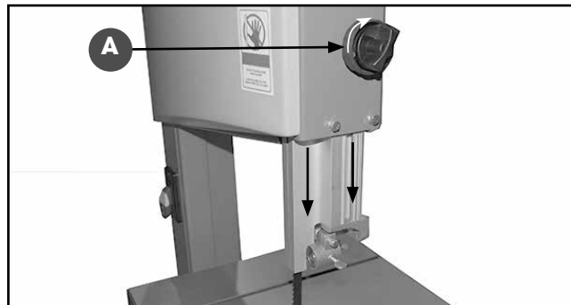
2. Lower the blade guard halfway by turning the knob A clockwise.
