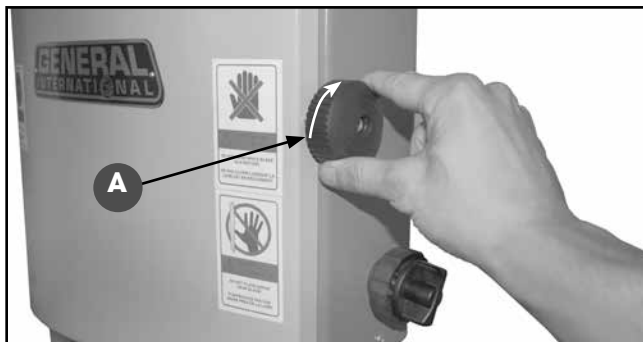
5. Open the upper door by turning the knob B clockwise.
