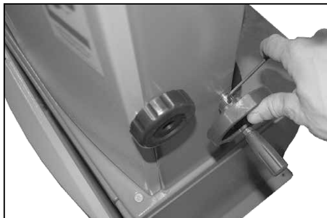
2. Secure the handwheel in place by tightening the set screw with a 3 mm Allen key.
