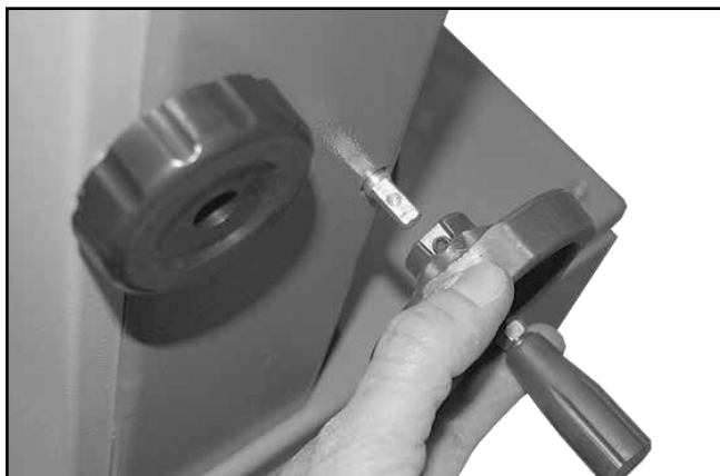
1. Slide the handwheel on the arbor.
