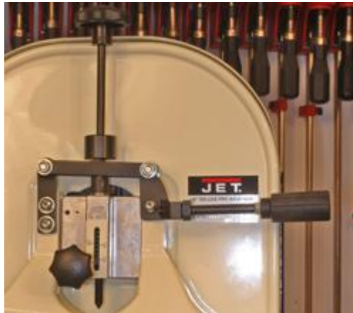
Blade tension adjustments and tension release (left) are easy to operate. The see-through window (right) in the upper door lets you monitor blade tracking changes with the doors closed!
