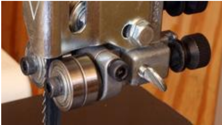
The JWBS-14DXPRO Band Saw features easy to adjust sealed ball bearing roller guides (left) above and below the table. The upper post is very rigid and moved up and down with a super smooth rack and pinion drive that has virtually no free play to make adjusting it perfectly for the material very easy.
