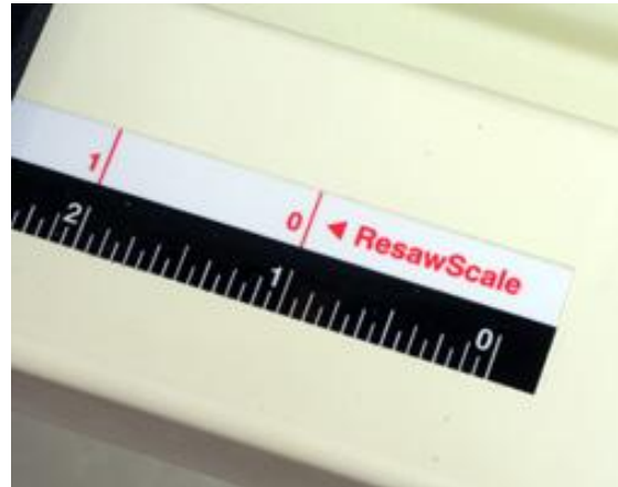
The scale on the fence rail shows both normal fence-to-blade markings but also has a second scale that shows blade to resaw post distance!
