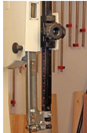
The JWBS-14DXPRO Band Saw features easy to adjust sealed ball bearing roller guides (left) above and below the table. The upper post is very rigid and moved up and down with a super smooth rack and pinion drive that has virtually no free play to make adjusting it perfectly for the material very easy.
