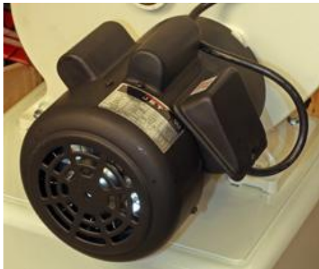
The motor is mounted directly to the lower saw enclosure (left). That mounting makes adjusting the belt tension or changing blade speeds (right) very easy.
