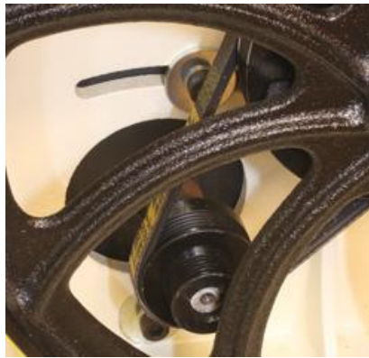
The motor is mounted directly to the lower saw enclosure (left). That mounting makes adjusting the belt tension or changing blade speeds (right) very easy.
