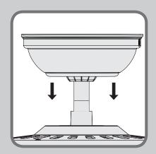
Remove the canopy. If uncertain how to remove it, reference the fan's owner's manual. With wiring exposed, it may be helpful to note existing wire connections or take a digital photo for reference. Remove the wire connectors that were connecting the wires from the outlet box to the fan, leaving the grounding wires connected.
