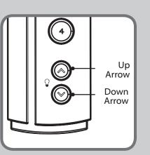
The up arrow and down arrow buttons control the lights on the fan. Quickly press the up or down arrow to turn the lights off and on. Hold the up or down arrow to raise and dim the light level.
