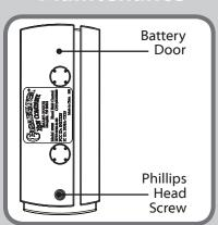
Installing or changing the battery -To access the battery compartment remove the small Phillips head screw that secures the battery door to the transmitter assembly. Replace with a CR2032 battery when necessary. The battery should be installed with the positive (+) side up.
