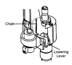
8. Place the bottom of the head through the lowering valve.
