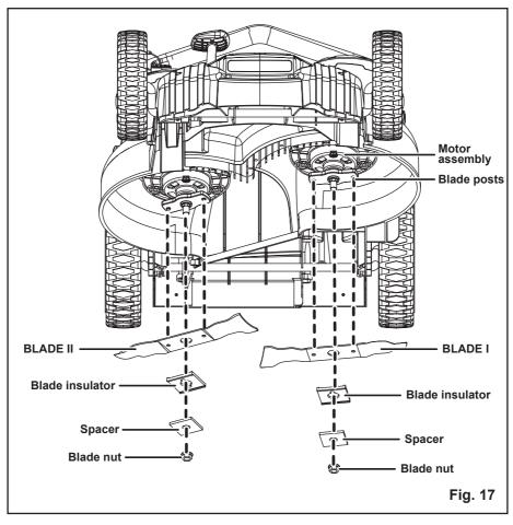
• Replace the blade insulator and spacer, then thread the blade nut on the shaft and finger tighten.
