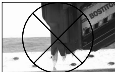
INCORRECT Placement of nail
