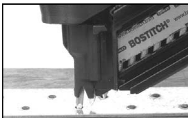
CORRECT Placement of nail
