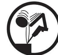
• Keep away from rotating end of tool. Do not wear jewelry or loose clothing. Secure long hair. Scalping can occur if hair is not kept away from tool and accessories. Choking can occur if neckwear is not kept away from tool and accessories.
