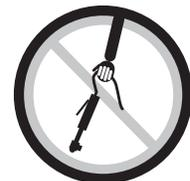
• Do not carry tool by the hose. Protect the hose from sharp objects and heat.
